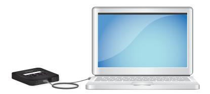
2. Connect the other end of the cable to an USB port on your computer or to the USB charger.
