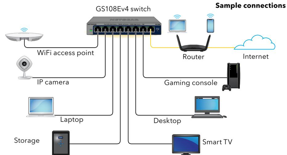
**NOTE:** We recommend that you use a Category 5e (Cat 5e) cable or higher-rated cable for Gigabit Ethernet connections.
