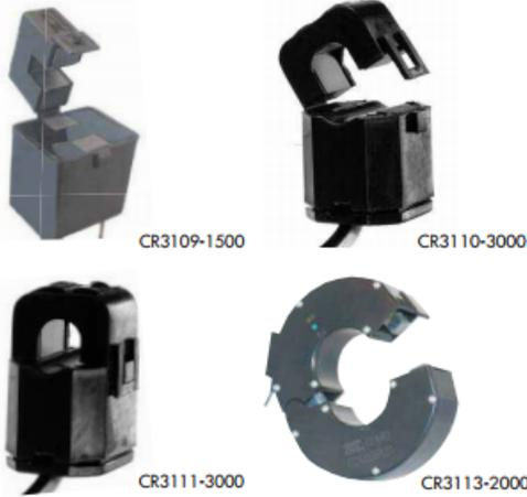
The **CR3100** Series Split Core Current Transformer is designed to provide a low cost method to monitoring electrical current. A unique hinge and locking snap allows attachment without interrupting the current-carrying wire. High secondary turn will develop signals up to 10.0 VAC across a burden resistor.
