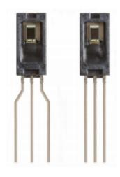
The HIH-4000 Series delivers instrumentation-quality RH (Relative Humidity) sensing performance in a competitively priced, solderable SIP (Single In-line Package).
