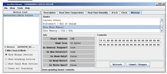
Figure 3: The MS-TH's four-digit type code being displayed in the first two available places. The first two digits, "19," are in the first spot and the second two digits, "01," are in the second.
