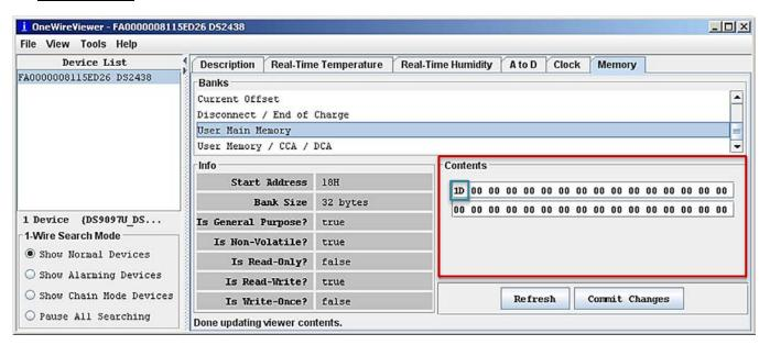
Figure 2: Under "Contents," highlighted by a red box, "1D" is being displayed in the first available space, highlighted by a blue box. This indicates that a MS-TW has been connected.
