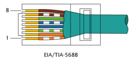
Figure 1: Standard EIA/TIA 568 RJ-45 Colors
