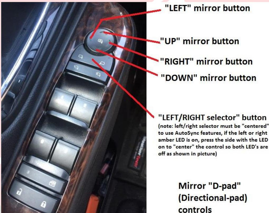
**-“DIESEL VEHICLES ONLY”-** Momentarily press the “LEFT” arrow of the mirror d-pad to activate the turbocharger boost pressure and Exhaust Gas Temperature display in the Driver Info Center (DIC). EGT is measured via the factory “EGT-1” sensor (turbo outlet for LML, downpipe pre-catalytic converter for
