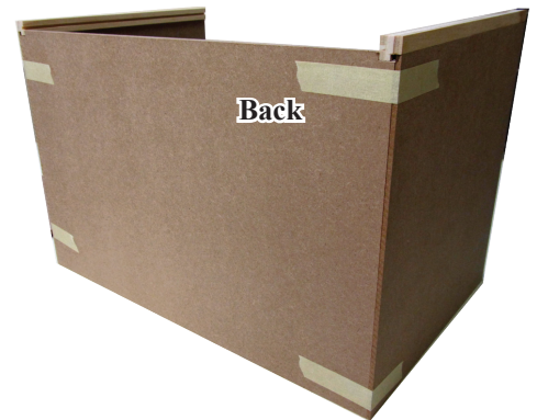
Stretch the tape for a tight glue joint
