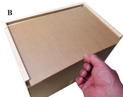
A little lift helps the Plexiglas go in the front groove
