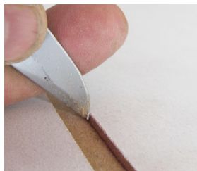
Cleaning a groove with a knife
