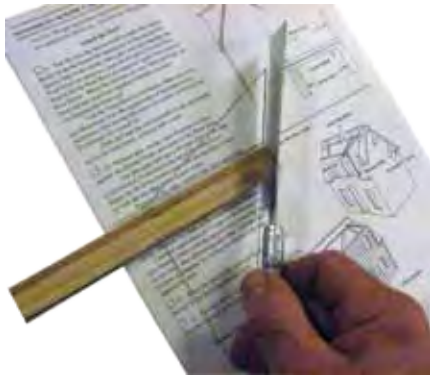
Use the pattern to cut the back angle
