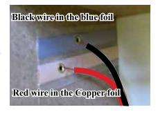
4. Tapewire: Poke a hole in each lead of the tapewire with the small (1mm) pin of the EL-66. Strip the ends of the connection wire and insert the ends into the hole. Push a small eyelet into the hole along-side the wire to stake the wire into the hole.
