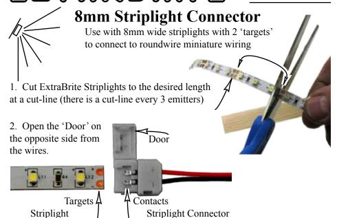
3. Slide the Striplight under the contacts so the contacts are centered on the targets.
