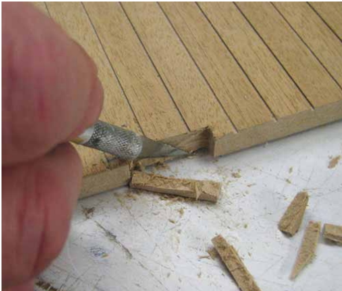
Cutting an Electrification Slot before building
