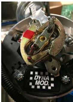
This Performance Distributors Street/Strip DUI unit will be used on our Blown Budget project engine in an upcoming story. It features a high-output coil and a vacuum advance canister for street use.
