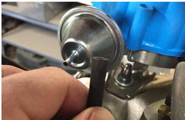
There's a tiny silver can on the side of most distributors that is easily the most misunderstood component of any distributor-based ignition system. Feared by many, and ignored by many more, the vacuum advance can is an important component of your ignition platform that offers both performance and economy. Leaving it unplugged is akin to throwing free engine efficiency straight down the drain.
