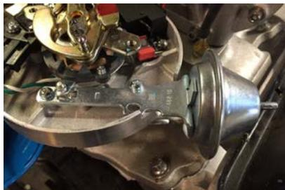
Here is the backside of the vacuum advance mechanism. Inside the can is a diaphragm that, when exposed to high manifold vacuum, pulls on a linkage to rotate the position of the reluctor tabs. When the source of vacuum dissipates, such as at WOT conditions, the advance returns to wherever it would normally be at that RPM.
