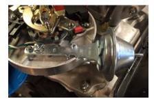
Here is the backside of the vacuum advance mechanism. Inside the can is a diaphragm that, when exposed to high manifold vacuum, pulls on a linkage to rotate the position of the reluctor tabs. When the source of vacuum dissipates, such as at WOT conditions, the advance returns to wherever it would normally be at that RPM.
