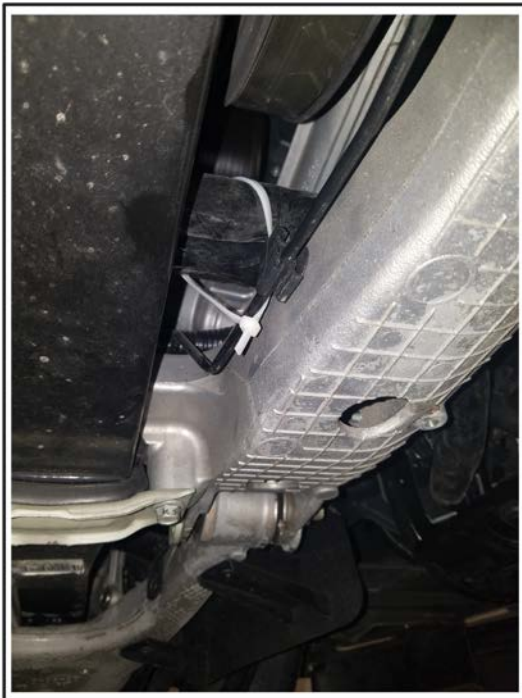
Figure 15 Oil hose routing
