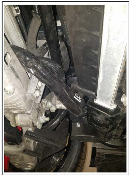
Figure 16 Oil hose routing
