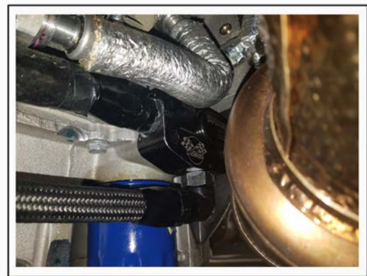
Figure 6 Oil Adapter with thermostat
