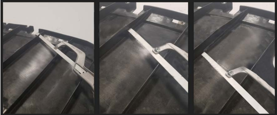
Figure 15 Air deflector modification. Remove the four (4) inner most ribs as shown
