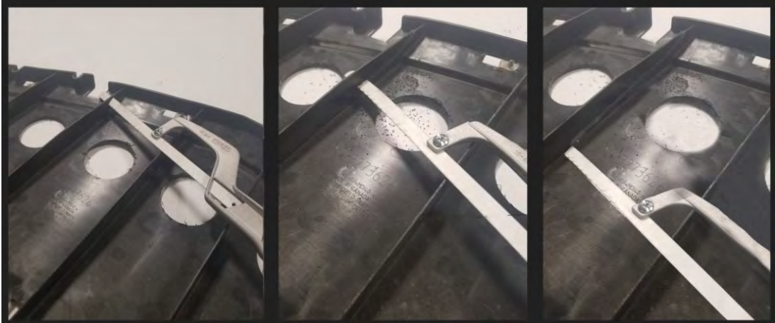
Figure 18 Deflector modifications Remove the four (4) inner most ribs as shown
