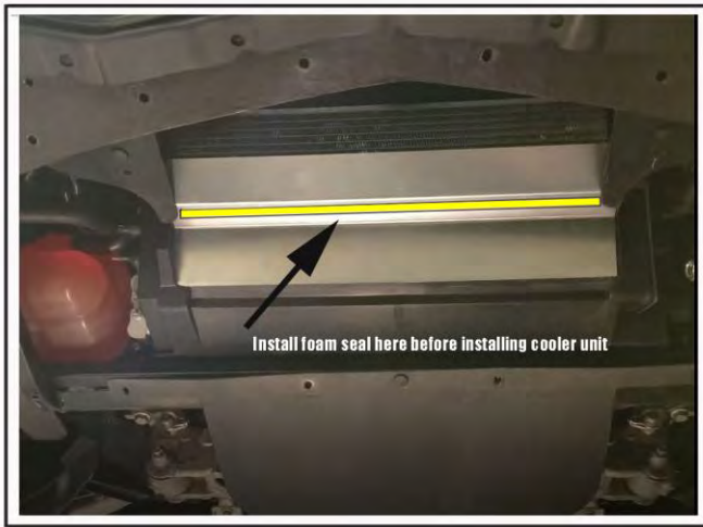
Figure 13 Finished cut out with air baffle installed
