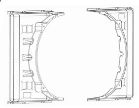
Connect the two halves by pushing them together until the interlocking tabs connect with each other and lock.
