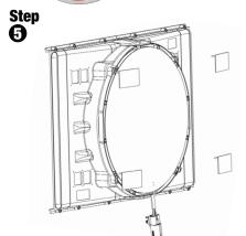
Install the four (4) rubber flaps, so they hang down, by piercing the pointed ends of the flap through the upper three (3) holes in the shroud. All four (4) flaps will use the upper mounting holes. Pull on the pointed ends with pliers until the flap fully seats against the shroud.
