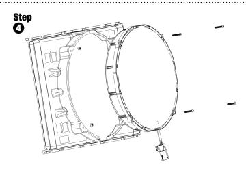
Attach a fan to the shroud using the four (4) 1/4"-20 x 1" button head cap screws with a washer on each one. Push bolts through the fan and into the shroud. Place flange nut on bolt from inside shroud. Torque to 90 in-lb.
