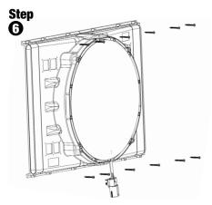
Using a self-tapping screw through each mounting boss, screw the shroud to the support (hat channel, extrusion) on the ends of the radiator with a #3 Phillips driver.
