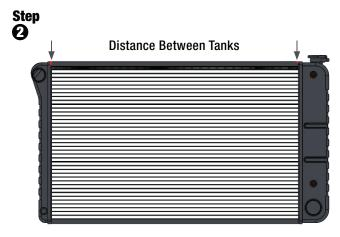
Measure your radiator in the flow direction between the tanks, then deduct 1/8" for shroud width.
