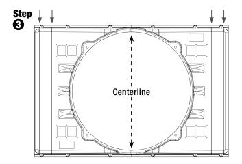
Center the radiator measurement on the shroud centerline. Note where your measurement ends in relation to the reference lines on the shroud. The lines molded in are for 22.5" and 26" wide radiators. Scribe your cut mark on the shroud and cut with a band saw, hack saw, or cutoff wheel.
