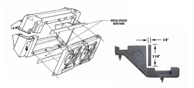
Enclosed with your radiator are two plastic aluminum spacer plates and hardware. Install these plates between the fan shroud and housing as shown, using the longer bolts supplied in the kit. This is required to prevent the fan shroud from damaging the thicker core. Also enclosed are the two self-adhesive foam seals. Stick one of the seals on the top of the radiator core and one on the bottom. Install the radiator as normal and reassemble the top cover with the modified cushions.
