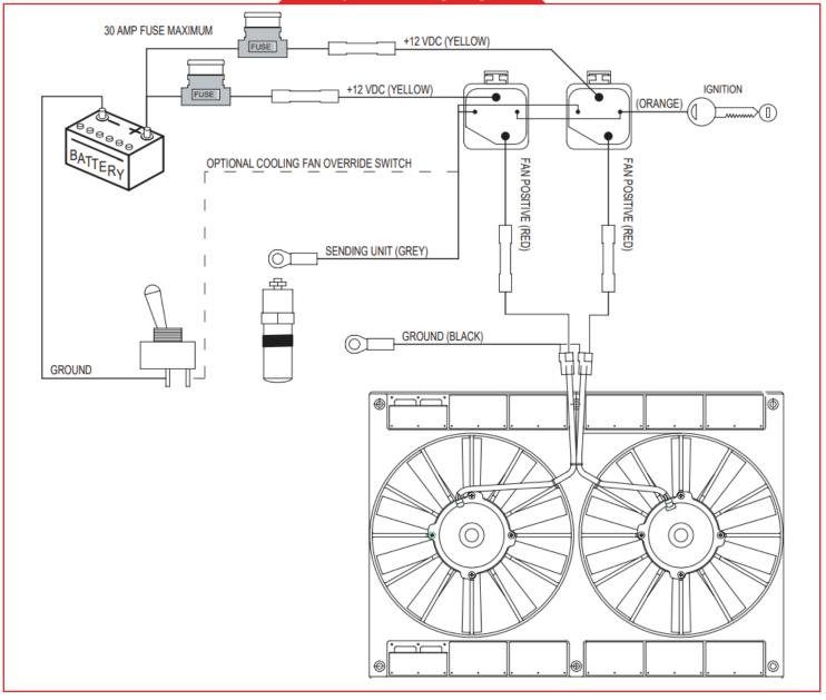
Air Conditioning requires a second relay. From the second A/C relay, connect Yellow and Orange wires to ground. Connect the Red wire to the sending unit wire of the original fan relay harness. The Gray wire from the A/C relay goes to the +12 volt A/C compressor clutch wire. The fan will turn on when the A/C compressor activates.
