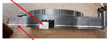
Cut back 1/2" all around the shroud. Leaving flanges on both left and right sides.
