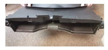
Finish cut along the bottom. You will cut through the foam seal on the bottom. Try to keep the remaining seal intact.
