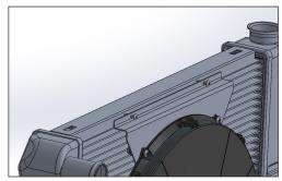
When the fan is resting in the channels, center the assembly how you wish.
