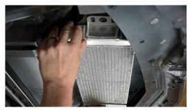
12. Place the paper template back over the cut area. Find the center lines of each hole and drill through each one with a 1/4" bit.
