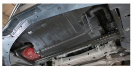
3. Locate the drain valve on the radiator. To eliminate unwanted spills, push a hose on the drain prior to opening and route the other end into a bucket for collection.
