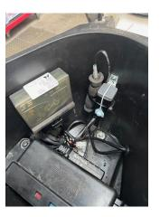
The **Setup Control Switch (2)** is hand held for setup of the speed limiter, and is then removed from the vehicle. This remains fitted to the vehicle when the cruise control is fitted, but there is a specific set of instructions that must be followed so that the speed limiter setup cannot be altered by the operator accidentally or intentionally.
