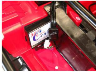
The **Setup Control Switch** (2) is hand held for setup of the speed limiter, and is then removed from the vehicle. This remains fitted to the vehicle when the cruise control is fitted, but there is a specific set of instructions that must be followed so that the speed limiter setup cannot be altered by the operator accidentally or intentionally.
