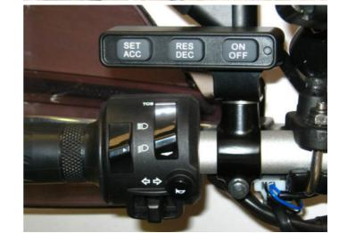
The standard **Control Switch (2)** mounts above the handlebar on the left side on the mirror mount. This switch has back lit buttons for night use, and an indicator light for power (ON-OFF) and engage indication.
