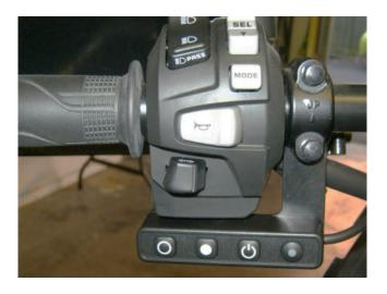
Optional alternate Switch Mounting Brackets (6 & 7) (see photos on the next page) are available for fitment on the right handlebar for DCT Shift bikes; these use the brake lever mounting clamp to mount the control switch. These brackets allow the control switch to be mounted either above (6) or below (7) the handlebar on the clutch lever clamp bolts. This mounting can also be used on Manual Shift bikes if necessary.
