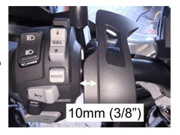
Another option for **DCT Shift bikes** is to mount the slim switch on the right handlebar between the bike's switch block and the brake lever mounting clamp. We don't usually recommend mounting the switch on the right side because holding the throttle steady while pressing the buttons on the cruise control switch is more difficult than using the switch on the left side, but this is a viable option for the slim switch.
