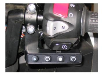
The same bracket is used for all these mounting positions, it is inverted to suit the mounting position above or below bar and on the left or right side.
