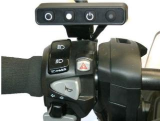
On Manual Shift bikes, our new Slim Control Switch (3) can be mounted on the left side handlebar, between the bike's switch block and the clutch lever mount. This switch also has backlit buttons for night use, and an indicator light for power (ON-OFF) and engage indication.
