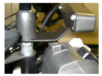
This photo shows the same switch and bracket mounted on a **DCT Shift bike**. This photo is from the previous model of the NC750X, but the switch mounting is the same as the manual shift shown above.
