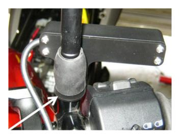
The optional New Slim **Control Switch (3)** mounts on the handlebar on the left side on the bikes' switch block. This switch also has backlit buttons for night use, and an indicator light for power (ON-OFF) and engage indication.
