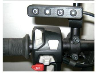
The Original Style Control Switch is also available with an optional shorter mounting bracket (4) also suitable for mirror mounting.
