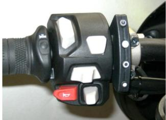
If the bike has mirror mounts built into the clutch lever, the **Original Style Control Switch with the taller mounting bracket** (3) is mounted above the handlebar on the left side on the clutch lever/mirror mount. This switch has backlit buttons for night use, and an indicator light for power (ON-OFF) and engage indication.
