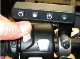
There is adequate space below the switch to use the controls on the bike's switch block when the above bar mounting bracket is used.
