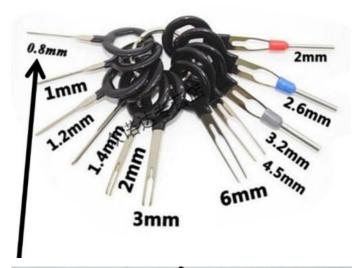
These sets have 3 or 4 single point tools usually. The finest tool in the set is the one needed.
