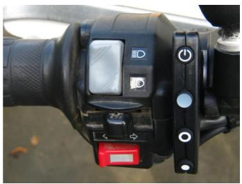
The optional **Standard Control Switch (4)** may be mounted above the handlebar on the left side on the clutch lever/mirror mount. This switch has back lit buttons for night use, and an indicator light for power (ON-OFF) and engage indication.
