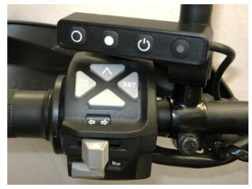
There is also another **optional switch mounting bracket available (3b)** that is mounted the same way, but positions the switch higher to allow easier access to the bike's switch block. As a result the angle the switch is set on can bring the switch closer to the rider for an easier reach to the switch.
