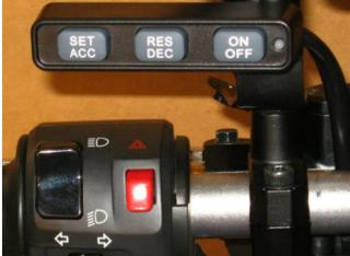
The Control Switch (2) is mounted on the left side mirror stalk.
