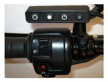
The alternative **Above Bar Control Switch (4)**. This bracket fits into the clutch lever handlebar mounting clamp. This places the switch lower and closer to the bike's switch block compared to the mirror mount. This switch mounting does not use the mirror mount. This mounting will not be available until the new control switch is released.
