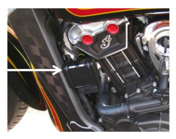
The photo above shows this **computer mounting bracket (2a)** below, which positions the cruise computer against the frame.
