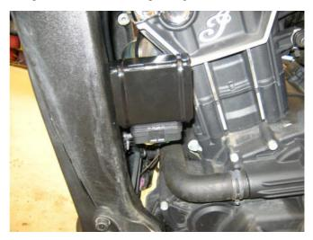
There is also a **computer mounting bracket (2b)** available for bikes fitted with crash bars that still uses the threaded hole in the frame. This bracket positions the computer away from the frame to allow space for the crash bar mount.
