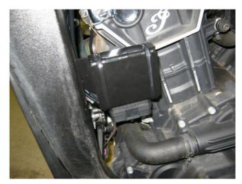
The bracket has a slotted mounting hole to allow for various designs of crash bars. The slot allows the computer to be moved in or out further from the frame so it can clear the crash bar mount. The closest gap possible with this bracket is roughly 20mm or 3/4" (photo below left), the largest gap possible is roughly 35mm or 1 3/8" (photo below right). This range should allow the cruise computer to be fitted with most, if not all crash bar mount designs.
