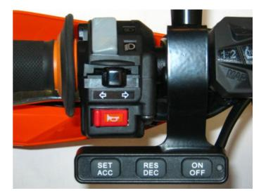
There is also **an optional switch mounting bracket available (5)** that places the switch below the handlebar.
