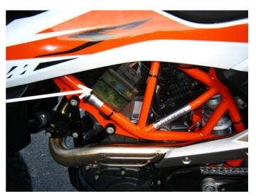
This photo shows the **Computer (1)** mounted on the KTM690 on a custom **bracket (2a)** on the left side of the bike, next to the motor.
