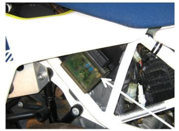
If the bike has the long-range fuel tank (the LR version) the computer and bracket on the previous page will not fit. We designed a new **bracket (2b)**. Either the **Standard (2a)** or **Long Range (2b)** bracket may be selected when ordering the cruise control. The Long-Range bracket will fit either version of the 701 Enduro.
