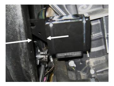
This photo shows a typical crash bar on a Scout, the mounting bracket above allows the cruise control computer to be fitted with this type of crash bar, using the same mounting bolt as the crash bar.
