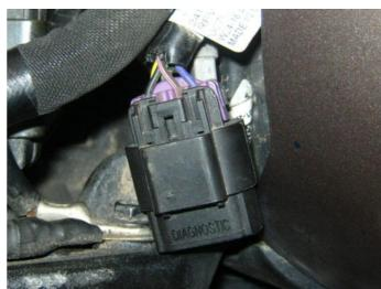
If the diagnostic plug has another plug fitted to it with wires coming out as shown here, you MUST purchase the CAN-BUS Dongle Patch with your kit, so that the cruise control AND the other device can both be fitted and connected to the bike's diagnostic plug.
