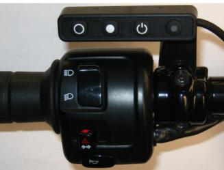
This **Below Bar Control Switch (6)**. This bracket fits into the clutch lever handlebar mounting clamp like the bracket above, but the switch is below the bike's switch block.
