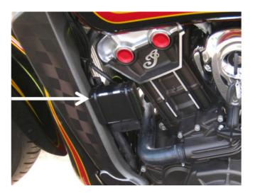
The photo above shows this computer mounting bracket (3a) below, which positions the cruise computer against the frame.
