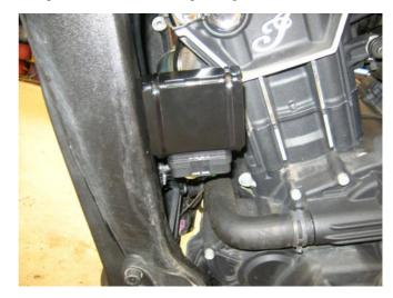
There is also a **computer mounting bracket (3b)** available for bikes fitted with crash bars that use the threaded hole in the frame. This bracket positions the computer away from the frame to allow space for the crash bar mount.
