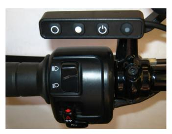
The alternative **Above Bar Control Switch (5)**. This bracket fits into the clutch lever handlebar mounting clamp. This places the switch lower and closer to the bike's switch block compared to the mirror mount. This switch mounting does not use the mirror mount. This mounting will not be available until the new control switch is released.
