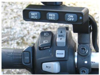
The **Optional New Slim Control Switch (3)** may be mounted on the handlebar next to the clutch lever mount. This switch also has back lit buttons for night use, and an indicator light for power (ON-OFF) and engage indication. This mounting location does make for a considerable reach to the cruise control switch.
