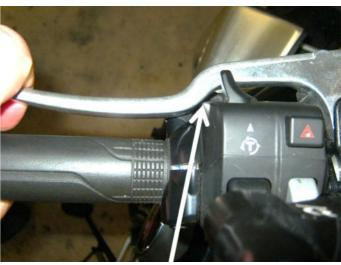
There is also an optional switch mounting bracket available (4) that places the Original Control Switch below the handlebar, however on this bike with the stock handlebars, there is not enough space between the handlebar and the fuel tank when the steering is turned full left. A gap of around 25mm (1") is required, and with the stock bars, the gap is around 18~20mm.
