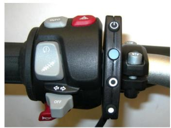
The optional **Standard Control Switch (3)** mounts above the handlebar on the left side on the clutch lever mount. This switch has back lit buttons for night use, and an indicator light for power (ON-OFF) and engage indication.
