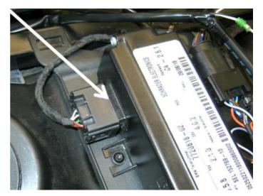
This photo at right, from another BMW model, shows the CAN-BUS plug connected to a blanking plug or 'Termination Plug' as it is known.
