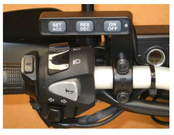
If you wish to mount the Control Switch (2b) below the handlebar, the switch bracket can be removed from the back of the control switch, turned over and re-fitted. Note that the handlebars may need to be rotated up slightly or risers fitted for this switch bracket to prevent the control switch contacting the fuel tank when the bars are turned full left. With the bars in the stock position, the switch may just contact the fuel tank on full left turn.
