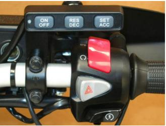
If you wish to mount the Control Switch (2d) below the handlebar, the switch bracket can be removed from the back of the control switch, turned over and re-fitted. Note that the handlebars may need to be rotated up slightly or risers fitted for this switch bracket to prevent the control switch contacting the fuel tank when the bars are turned full right. With the bars in the stock position, the switch may just contact the fuel tank on full right turn.
