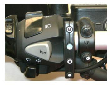
Another option is the Slim Control Switch Below Bar (3b) mounting is this bracket that mounts the control switch below the bike's switch block.
