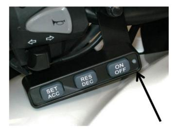
For below handlebar mounting the bracket mounts between the lower faces of the clamp. The clamp must have about  $1\sim1.5$ mm (0.040" $\sim0.060$ ") filed from the lower face of the clamp to allow for the thickness of the switch bracket.
