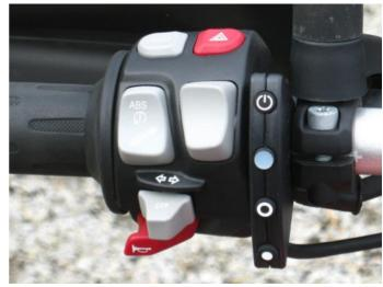
The optional **Standard Control Switch (3)** mounts above the handlebar on the left side on the mirror stalk mount, however the standard brush guards cover the mirror mount so this will NOT fit with the original brush fitted to the bike. This photo is from an earlier model F800GS where the brush guard mounting was different. This switch has back lit buttons for night use, and an indicator light for power (ON-OFF) and engage indication.
