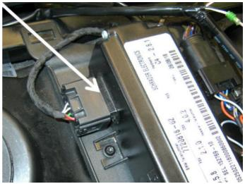
NOTE: - If you purchase the dongle patch, and connect it to the bike's blanking plug, this may degrade the signal enough to prevent the cruise control operating. Leaving the plug disconnected is not recommended, as having an un-terminated (disconnected) plug on a CAN-BUS circuit can cause errors with the bike's communications systems.
