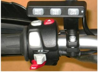
The current model F800GS has hand guards on the handlebars and the mount for the hand guard covers the mirror mount. This makes it impossible to fit a switch mounting bracket to the mirror mount, the hand guard mount covers the mirror mounting boss on the clutch lever/mirror mount.
