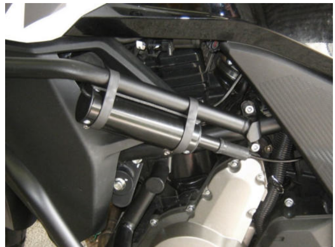
Servo mounted below the crash bar.
