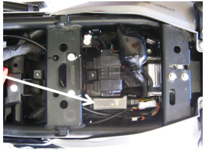
Servo mounted below the crash bar.
