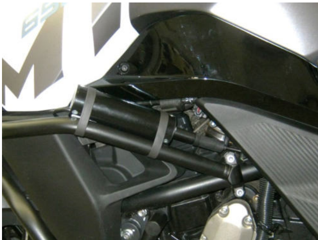
Servo mounted above the crash bar.
