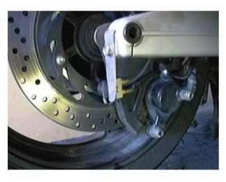
The **Optional Wheel Speed Sensor (8)** is mounted on the end of the right hand side of the swing arm under the axle pinch bolt. Nickel plated magnets are placed in the heads of the bolts that mount the brake disc. **NOTE: - Not all models need this, see the last pages of this document for details.**
