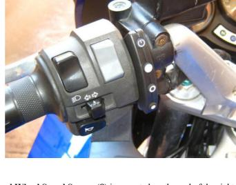
The new **Slim Control Switch (7)** is also available for this model. This switch mount directly on to the handlebar between the bike's switch block and the clutch lever mount.
