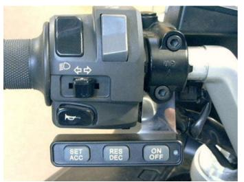
An alternative mounting for the **Control Switch (6)** is available so the switch is mounted below the handlebars. The bracket mounts between the bottom faces of the clamp and the master cylinder. The clamp must have about  $1\sim1.5$ mm (0.040" $\sim0.060$ ") filed from the bottom face to allow for the thickness of the switch bracket.
