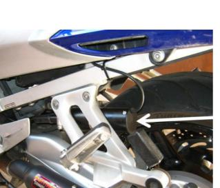
The Electric Throttle Servo (2) is mounted inside the left side passenger's footrest 'hanger'.
