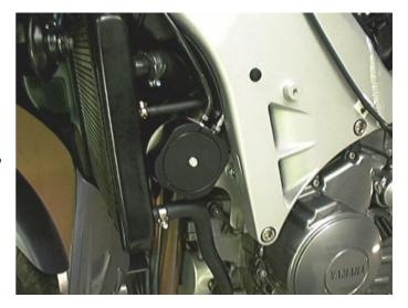
The **Control Switch (5)** can be mounted to the left hand (clutch) master cylinder handlebar clamp. The bracket mounts between the top faces of the clamp and the master cylinder. The clamp must have about  $1\sim1.5$ mm (0.040" $\sim0.060$ ") filed from the bottom face to allow for the thickness of the switch bracket.
