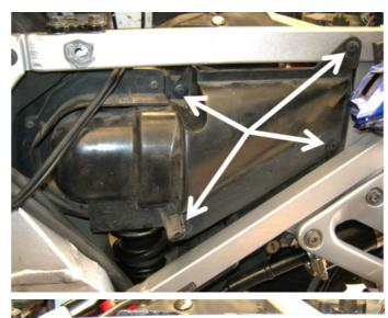
• Under the cover is the engine ECU connector. This is a sealed 44-way plug.
