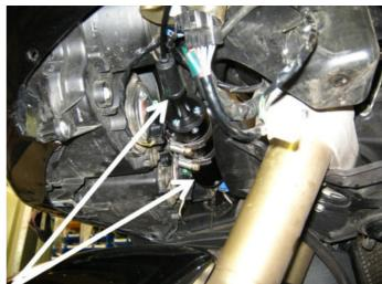
The Cable Interface Unit (3) is located on the left side of the motor, near the front left corner of the engine. It has a new cable (4) running from it to the fuel injection throttles. The photo shows the CIU with the fairing fitted to the bike. The CIU is mounted below the crash knob.
