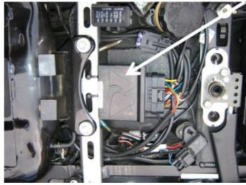
The **throttle servo (2)** mounts behind the headlight using the headlight mounting screws. The photo is taken looking up from low on the left side of the bike.
