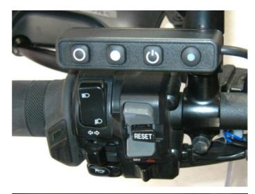
The New Slim **Control Switch (5b)** mounts on the handlebar on the right side on the bikes' left switch block. This switch also has back lit buttons for night use, and an indicator light for power (ON-OFF) and engage indication.
