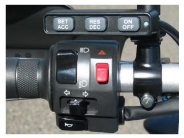
The New Slim **Control Switch (5b)** mounts on the handlebar on the left side on the bikes' switch block. This switch also has back lit buttons for night use, and an indicator light for power (ON-OFF) and engage indication.
