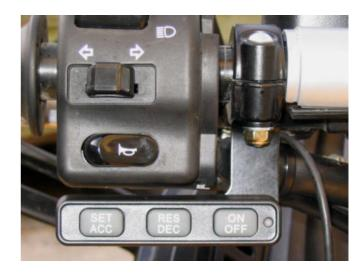
On the SE5 (electric shift model) the **Control Switch (6E)** is mounted on the clamp for the paddle shift switch assembly. Approximately 1.5mm must be filed from the inside face of the clamp bracket for the shift switch to allow for the thickness of the cruise control switch bracket. This is clamp bracket NOT part of the shift switch, but a separate clamp to hold the switch mechanism to the handlebar.
