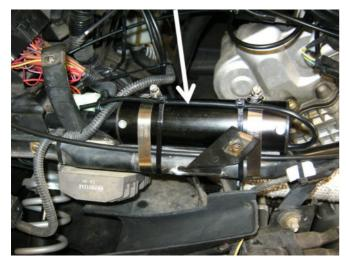
The Cable Interface Unit (3) is located above the front cylinder head on the engine. A new cable (4) connects it to the throttle bodies.
