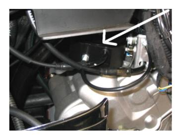
The **Speed sensor (5)** is mounted on the right side of the swing arm, on one of the inner fender mounting bolts. Nickel plated magnets are placed in the heads of the bolts that mount the ABS tone wheel.
