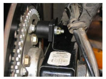
The **Electric Throttle Servo (2)** is mounted to the frame on the left side of the bike, to the left of the engine.
