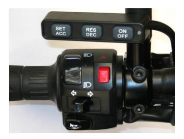
We also offer an alternate mounting bracket (5b) to mount the switch below the handlebar. This is offered at no extra cost at time of ordering, or the switch bracket may be purchased at any time.
