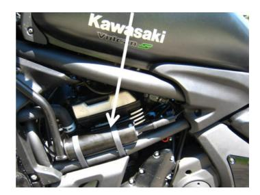
The plastic frame cover panel must be 'notched' to allow for the servo cable.
