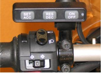
An alternate bracket is available to mount the **Control Switch (5b)** above the handlebar on the mirror mount, but it is lower, about 10 mm (3/8") above the bike's switch gear.
