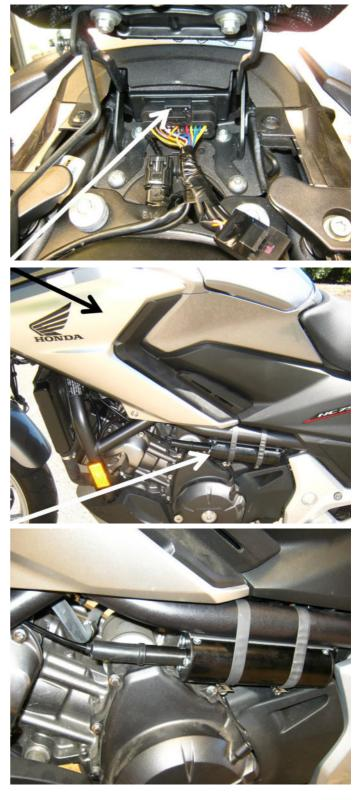
The CIU (3) is mounted on the front of the air filter housing using Velcro mounting tape. A new cable (4) connects it to the throttle bodies.
