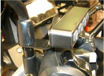
The **Control Switch (6)** may also be mounted this way on the DCT version of the bike. These photos show an earlier version of the switch fitted to a Honda CTX700 which has similar switch gear. The control switch does not interfere with operation of the park brake.
