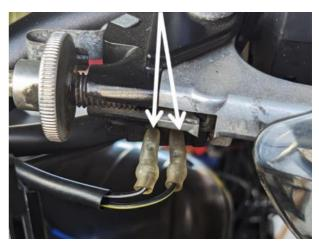
For the 2017 model year, a new type of clutch switch is fitted that has a two-way latched plug. The switch is located directly under the clutch lever near the pivot point. This connector (arrowed in the photo below left) comes from the rear into the clutch switch. Cruise control MCS 6740/2 will fit these bikes.
