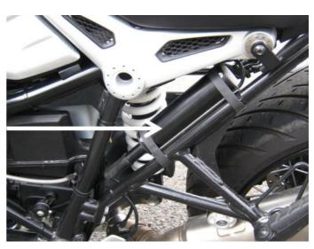
The bike's original throttle cable splitter box (throttle cable divider) is removed from the bike and our **Cable Interface Unit (3)** is fitted to the bike. No modifications to the bike's cables are required at all, it is a straight swap.
