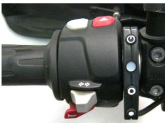
The standard **Control Switch (4b)** mounts above the handlebar on the left side on the mirror mount. This switch has back lit buttons for night use, and an indicator light for power (ON-OFF) and engage indication.
