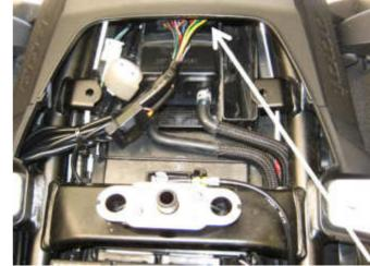
The **Electric Throttle Servo (2)** is mounted on the left side of the engine.
